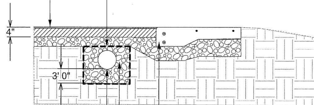
4 INCH PERFORATED PVC DRAIN PIPE PITCHED
